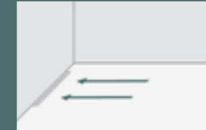
Drain positioned against the short wall
