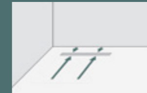
Drain positioned off the wall
